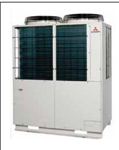
Mitsubishi's Q-ton air-to-water CO<sub>2</sub> heat pump has a COP of 4.3 and can be installed in hotels, care homes, leisure centers, and other building applications.<sup>122</sup> The Q-ton has the ability to maintain high capacity, particularly in cold conditions and has a capacity of 30 kW, generating hot water up to 90°C (194°F).<sup>123</sup> The system can maintain 100 percent capacity even when temperatures reach -7°C (19°F), and when temperatures reach -25°C (-13°F) the
